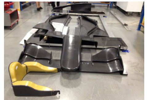
The front wing assembly (foreground) is much like the one used in the IndyCar Series; the underwings (rear) come in two pieces. (Photo: Curt Cavin/The Star)
